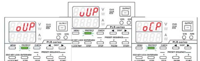
OVP (Over Voltage Protection) UVP (Under Voltage Protection) OCP (Over Current Protection)
