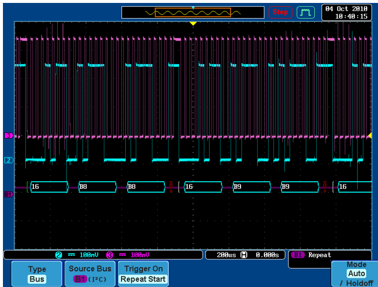
Fig. 7 Illustration of the GDS-3000 I 2 C decoding
